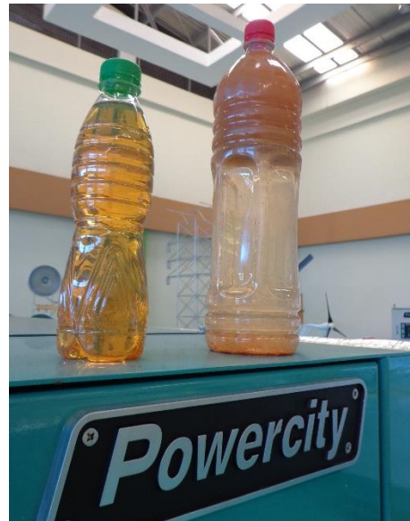
Bottle on the left contains clean and fresh diesel. Bottle on the right contain oxidized diesel (upper part) and contaminated with free water and sludge (lower part).
