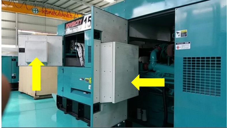
An example of Powercity generator set with aluminum encased fiberglass sound absorber fitted in NEMA enclosure.
